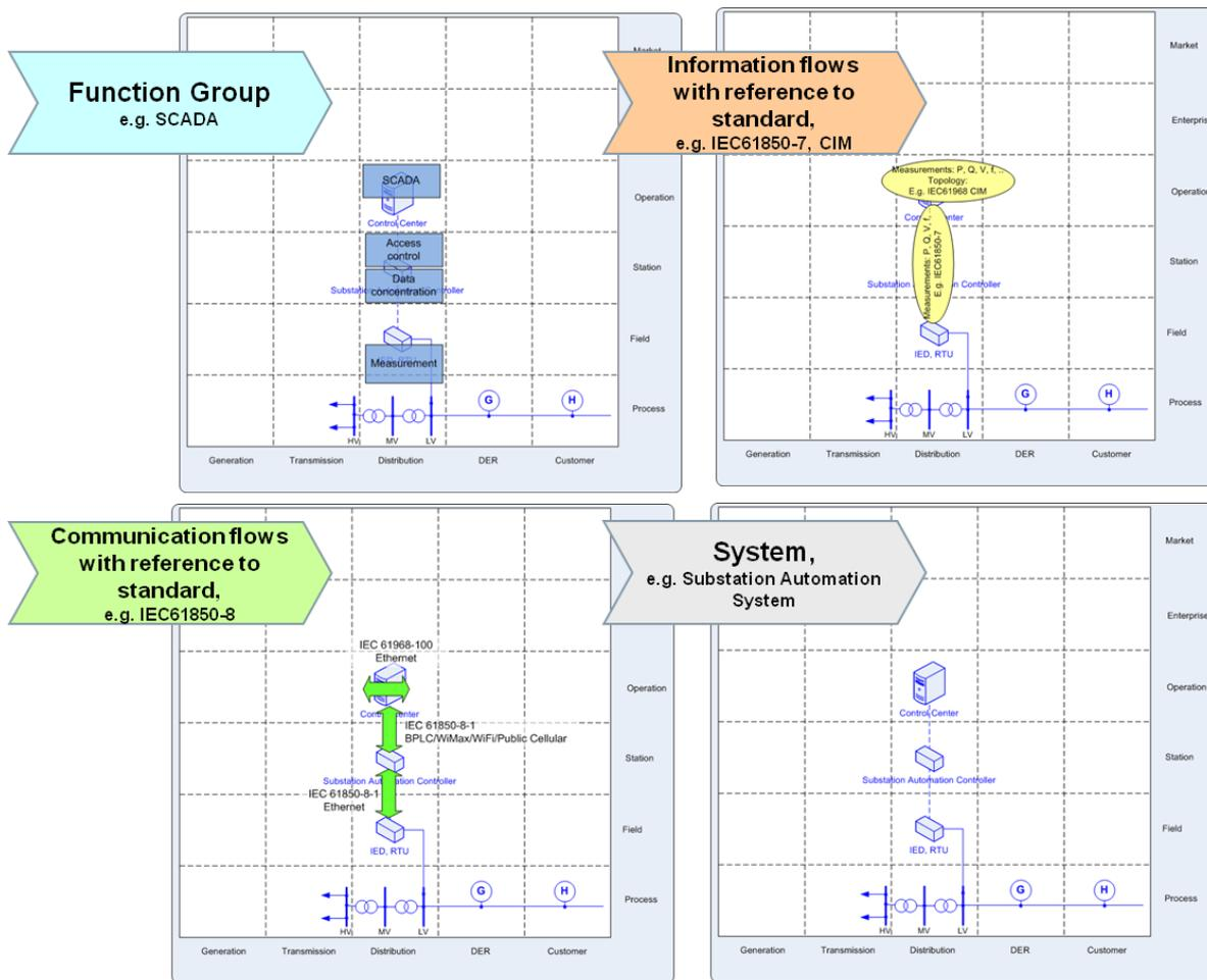
Figure 22: SGAM analysis for “Monitoring inside the distribution grid”
