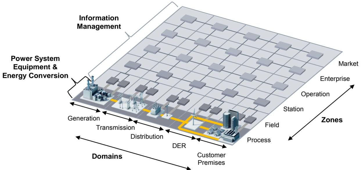
Figure 1: Smart Grid Plane – Domains & zones of SGAM
